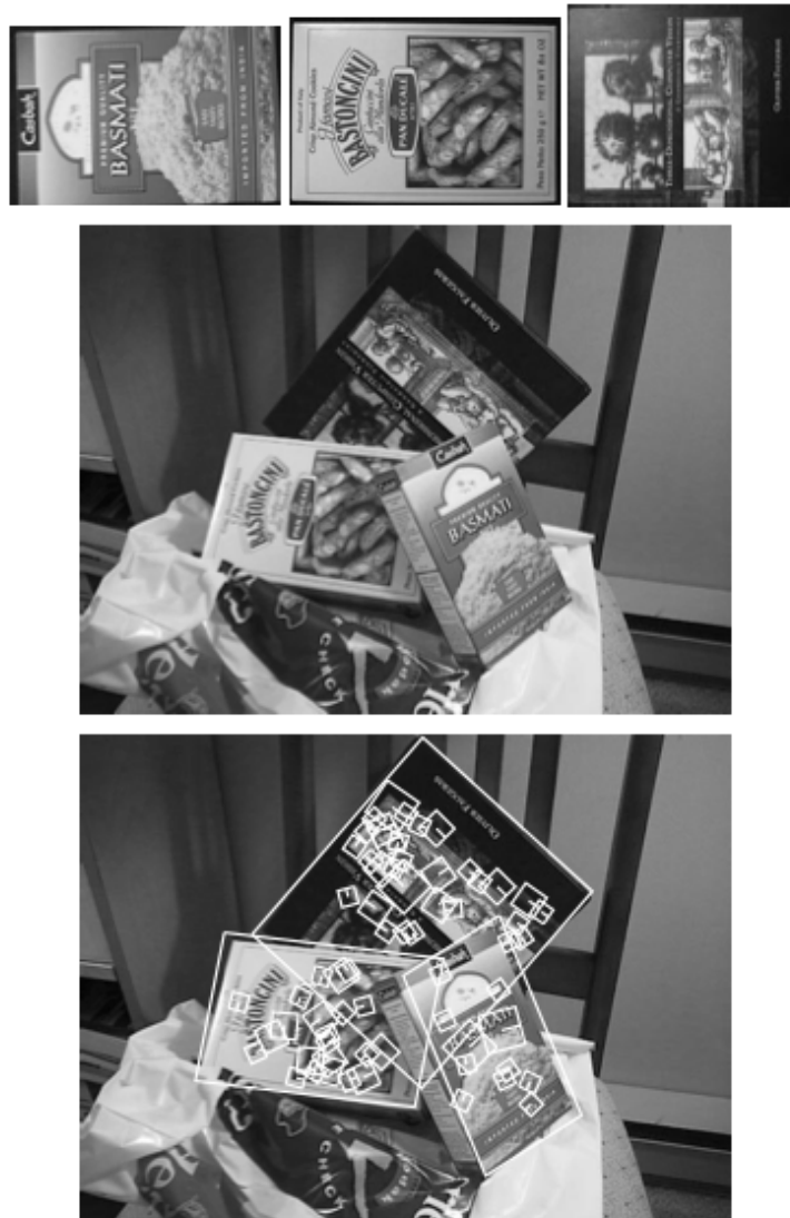
Fig. 28.1 The SIFT algorithm finds keypoints in an image, i.e. localized features that are particularly useful for identifying the objects in an image. The top row shows images that are matched against the image in the middle row. The bottom-row image shows some of the keypoints used to perform the matching (i.e. these keypoints demonstrate the same features in the top-row images and their transformed middle-row counterparts). SIFT keypoints are identified via a staged filtering approach. The first stage identifies key locations in scale space by looking for locations that are maxima or minima of a difference-of-Gaussian function. Each point is used to generate a feature vector that describes the local image region sampled relative to its scale-space co-ordinate frame. The features achieve partial invariance to local variations, such as affine or 3D projections, by blurring image gradient locations.
