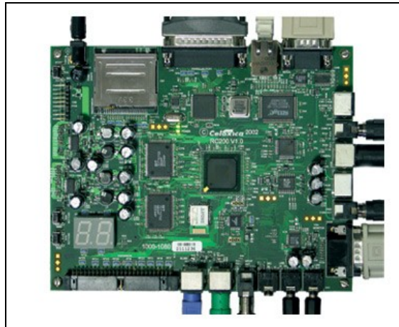
Fig.1. The Celoxica Board with central FPGA
