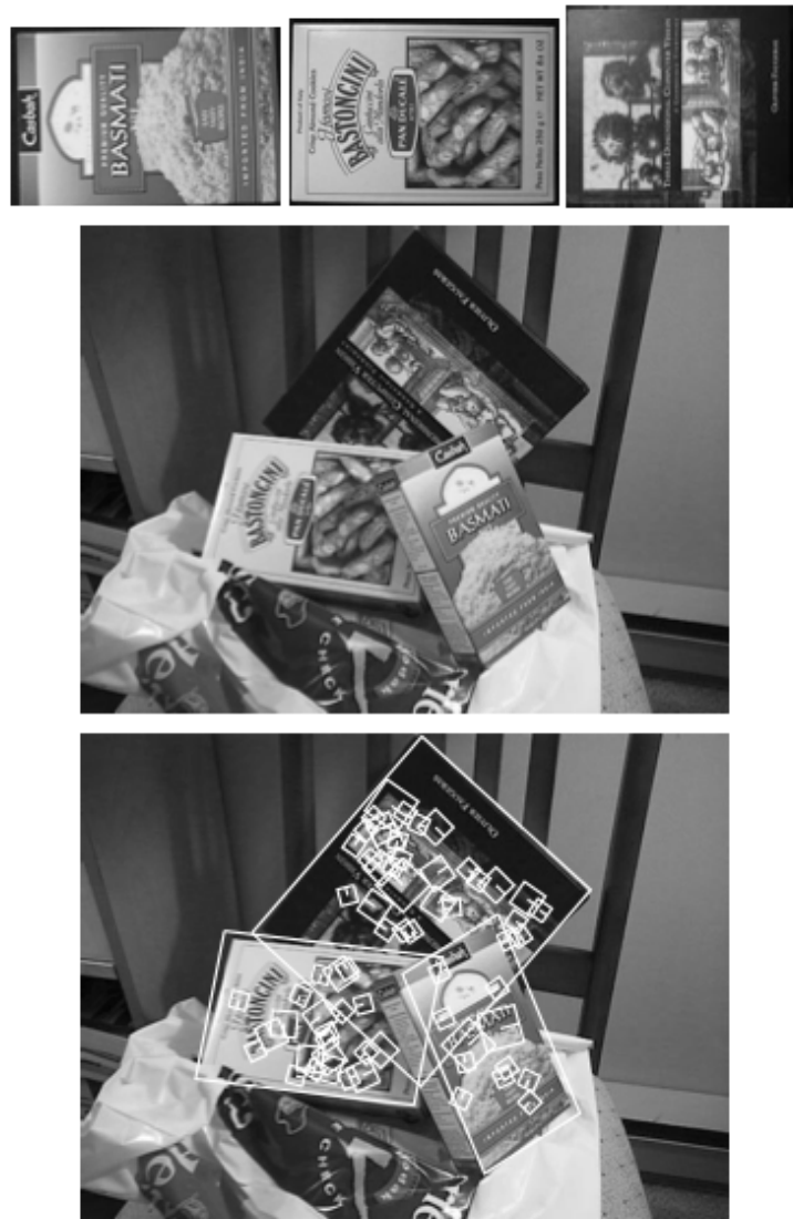
Fig. 1. The SIFT algorithm finds keypoints in an image, i.e. localized features that are particularly useful for identifying the objects in an image. The top row shows images that are matched against the image in the middle row. The bottom-row image shows some of the keypoints used to perform the matching (i.e. these keypoints demonstrate the same features in the top-row images and their transformed middle-row counterparts). SIFT keypoints are identified via a staged filtering approach. The first stage identifies key locations in scale space by looking for locations that are maxima or minima of a difference-of-Gaussian function. Each point is used to generate a feature vector that describes the local image region sampled relative to its scale-space co-ordinate frame. The features achieve partial invariance to local variations, such as affine or 3D projections, by blurring image gradient locations.
